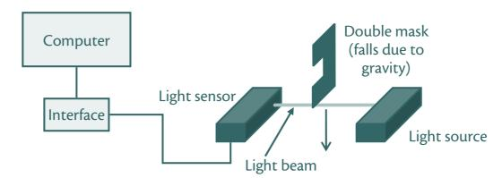
The double mask is used to interrupt the light beam and send a signal to the computer. The computer measures the initial speed u, the final speed v, and the time interval t. It then calculates the acceleration a using the formula:
