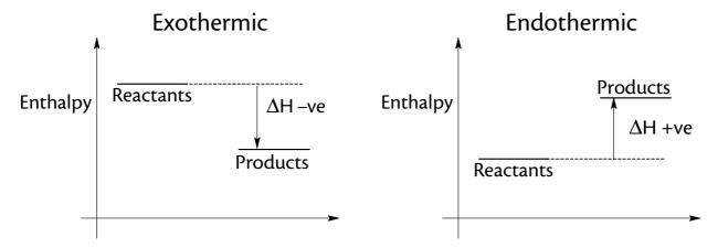
Exothermic Reactions: If, in the process reactants to products, the chemicals release some of their enthalpy in the form of heat then the products must have lower enthalpy. It stands to reason that  $H_p - H_r$  must be negative, (ie  $\Delta H$  is -ve).
